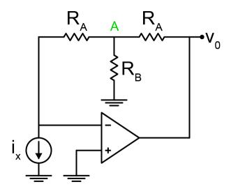
Derive an expression for the output voltage  $v_0$  in terms of the input current  $i_x$ . Then select values for  $R_A$  and  $R_B$  in the above circuit so that the output voltage is approximately
