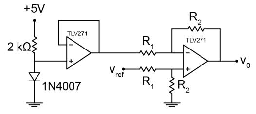
The tunable input voltage  $v_{ref}$  should be chosen to subtract the offset voltage, and the resistors  $R_1$  and  $R_2$  should be selected from the values available in your kit, to achieve the desired scale ratio. Do not use any resistors in your design that are smaller than 1 k $\Omega$  in size.
